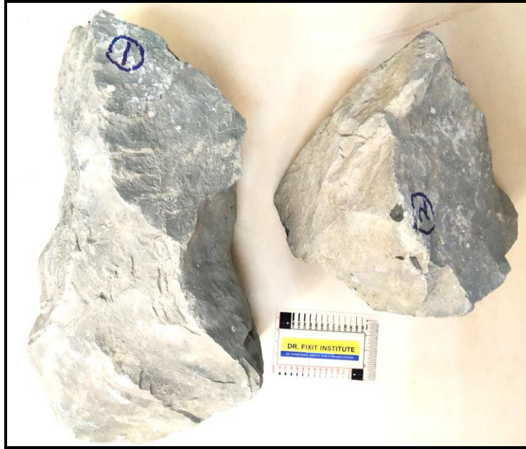
Figure-1: Photograph showing particles of rock boulders with crystalline surface texture
